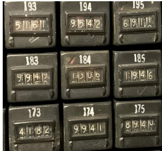
Some of the peg count registers from our 1923 Panel switching system
