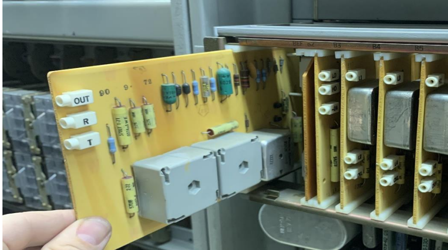
The transistorized DTMF decoders in the senders of the museum's No. 1 Crossbar system
