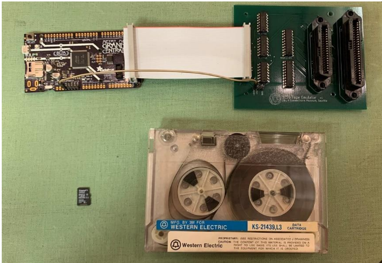
The drive emulator that Colin Slater built, and a faulty tape cartridge.
