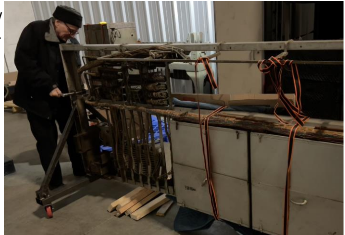
A homemade device permits easier and safer moving for heavy panels
