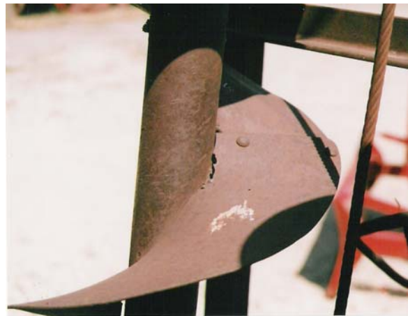
Detail of the bolted-on cork-screw of the well casing auger.
